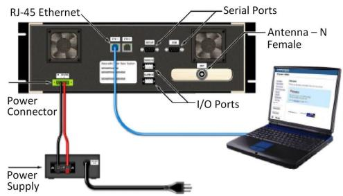
Connect an Ethernet cable to the first LAN port of the Viper SC+ and connect the other end into the Ethernet port of your PC.
